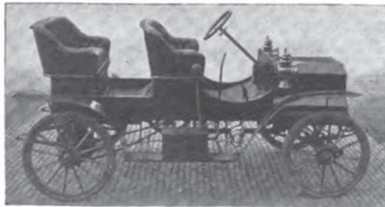
The "Overholt" Air-cooled, Friction Drive Motor Surrey. Price $650. Also furnished as a single seat runabout at $600.
